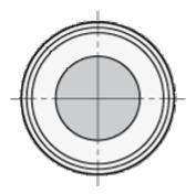
$\begin{array}{ll} d1 & = 25 \\ d2 & = 22 \\ h & = 8.5 \\ Holding force N = 14 \end{array}$
